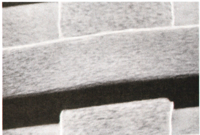
Fig. 1. Resist step coverage: 1- \mu\text{m} -thick resist pattern over 0.5- \mu\text{m} -high step.
